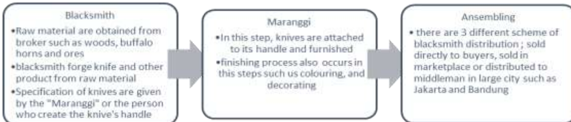
Figure 6. Blacksmith Industry Process
